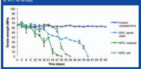
Figure 2. Tensile strength changes of PLA incubated in compost, soil and sterile water at 50°C for 60 days
