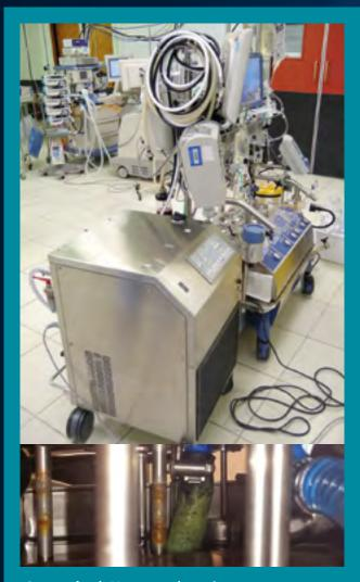
Figure 1 (top) Heater-cooler unit Figure 2 (bottom) Biofilm growth on the internal components of the heater-cooler
