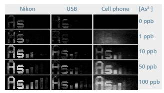
Microfluidic encapsulation-enabled microbial sensor array for monitoring arsenic contamination, showing different output patterns on various arsenic (As<sup>3+</sup>) levels. Left, middle, right panels: images acquired by a Nikon microscope, USB fluorescence microscope and cell phone camera.
