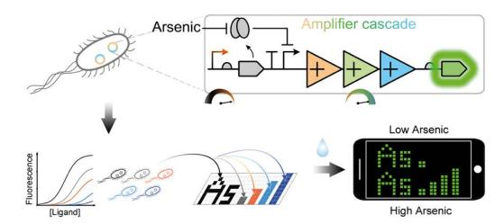
A microbial sensor array displaying an easy-to-read volume bar-like pattern for mobile phone-based field monitoring of arsenic contamination.
