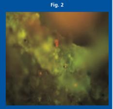
A composite EDIC/fluorescence image of the surface of a drinking water pipe. Cells of L. pneumophila have been labelled with a PNA probe with a red fluorophore attached. Magnification x 1000
