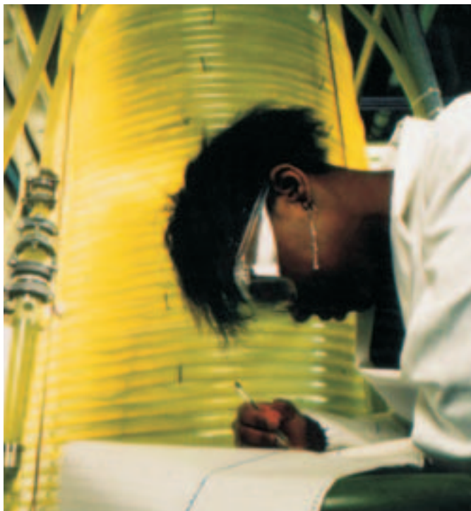
Figure 3. 230 litre tubular flow bioreactor for culturing microalgae
