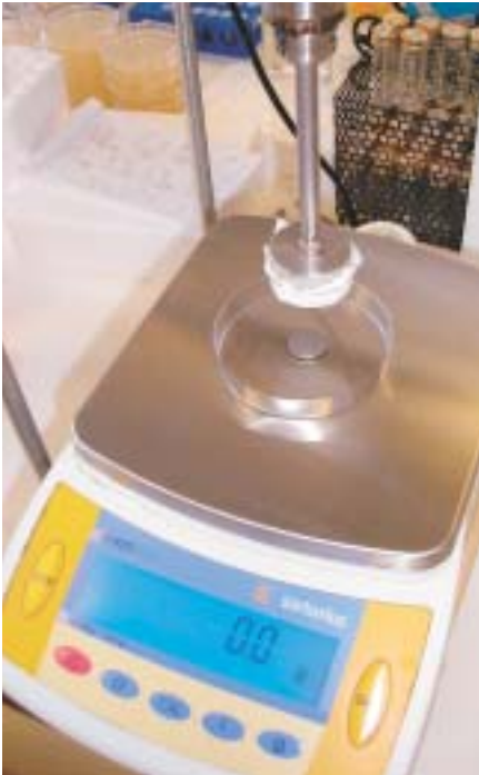
Figure 1. Step-1 of the new protocol examining the ability of disinfectant wipes to remove microbial contaminants from surfaces. Wipes are placed in contact with surfaces and mechanically rotated.
